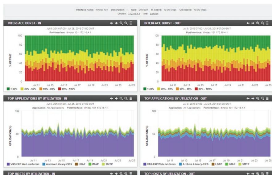
Figure 2: View utilisation levels over time and investigate who and what is making links busy.
